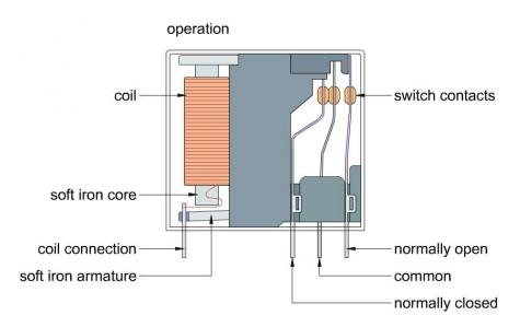
You may see that the common terminal and the normally closed terminal have continuity When the coil of the relay is at rest.
